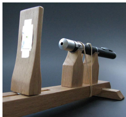
Figure 2-2. The basic set up for a stand to measure the power of a lens using a laser..
