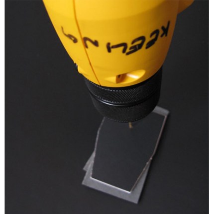
Figure 1-2. Drill a light path in both cardstock and posterboard at the same time using a 1/16 (or smaller if you have one) bit.
