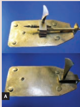
Fig. A: Brass replica of a van Leeuwenhoek microscope (front and back views). You can build one from simpler materials, with the same optics and operating principles.
